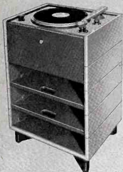
BQ-1A TURNTABLE. For fine-groove 45's and 33 1/2 LP's (exclusively)—up to 12". Only 28" high, 20" wide, 16 1/2" deep, this studio-proved unit is your answer for a moderately priced turntable. Complete, with lightweight tone arm, filter, 1.0 mil pick-up, and cabinet.
